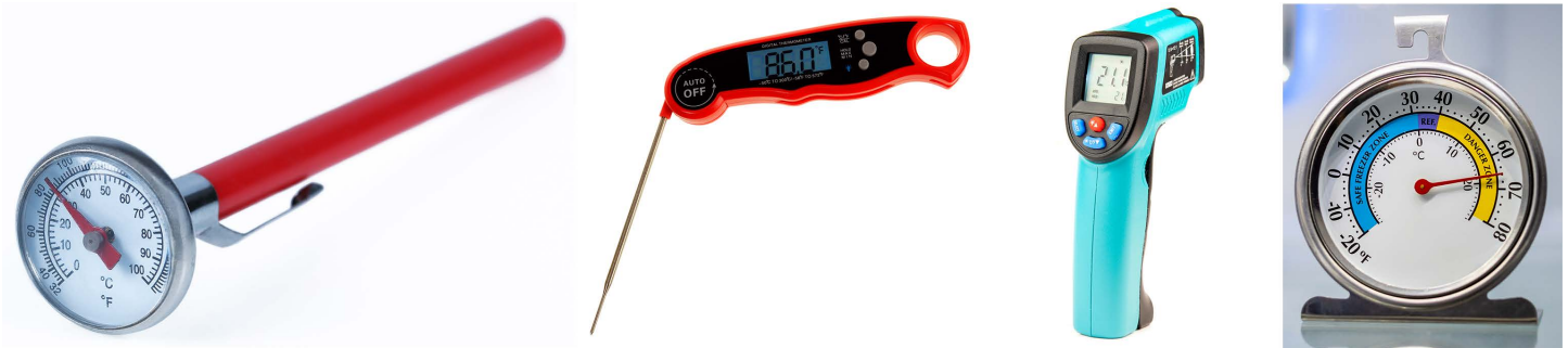
Commonly used thermometers, Left to right: Bimetallic stemmed thermometer, general purpose use; Digital Thermometer, general purpose use, popular due to its instant-read capabilities; Laser or Infrared, best used for measuring equipment temperatures because it only provides a surface reading; Air Temperature Thermometer, generally used inside refrigeration equipment
